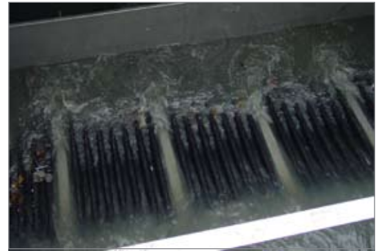
Continuous backwashing action cleans debris from screens.
