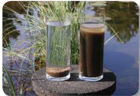
SVI5 comparison of aerobic granular sludge (left) and conventional activated sludge (right)
